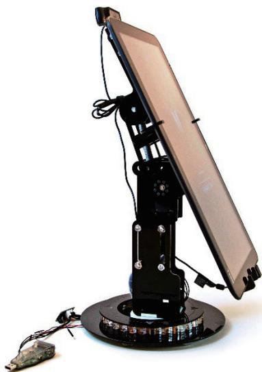
Figure 2. Jarvis: A desktop pan & tilt telepresence robot equipped with an 18" screen and HD video camera.
